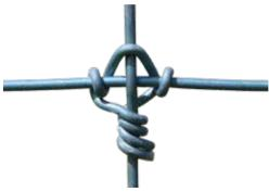
The prefabricated fence wire design is favoured for longer spans and suspension fence designs. The single picket wire has a "dropper" effect and creates a stiffness in the fence, whilst the knot allows for some movement of both the picket and horizontal (line) wire. This unique feature allows the fence to absorb impact and spread load. Available with or without preattached 30cm hinged apron.
